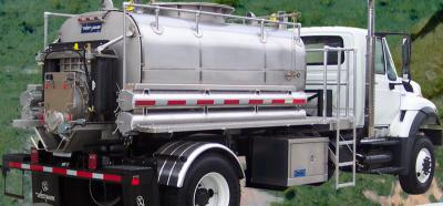
4x2, 4x4, 6x4, or 6x6 Chassis: Capacity: 1000 - 3000 Gallons Various Available Shape: Material: Stainless Steel or Aluminum
